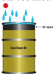
If the drum is placed outside, rain or snow settles on top of the drum.
