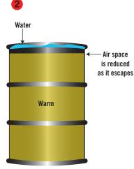
When the surrounding area's temperature rises, the oil expands and air in the drum escapes.
